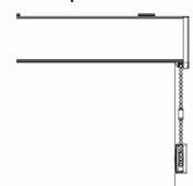
B. System 40® standard metal bracket top front view.
