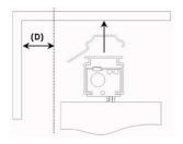
Measure and mark the distance (D), allowing for obstructions like handles that protrude into the recess area. Hold the blind in the recess and find the bracket fixing position. Drill brackets into position 5cm from the recess side walls.
