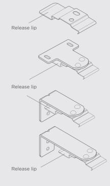
Mark the hole positions before drilling and plugging if necessary. Use two screws in each bracket ensuring that the brackets are level. Remember to allow room for the blind to clear any obstacles when deployed, e.g. door or window handles.
