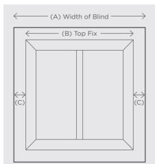
outside the window ensure that FIXING. To calculate C (A-B)/2.
