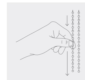
Repeat step 2 pulling chain in the opposite direction until travellers are fully aligned.
