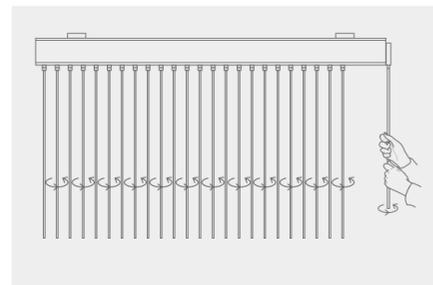
If any of the slats are out of alignment, twist the wand control until the slats are in the closed position, then continue to twist the wand until all the slats are fully aligned. **You may feel some resistance and hear a clicking noise whilst doing so.**
