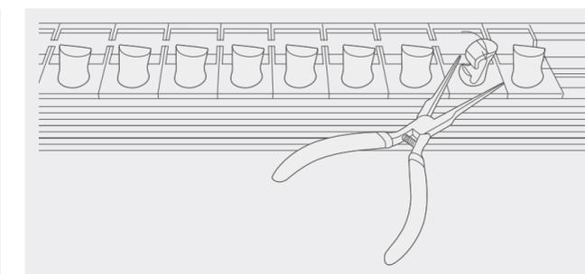
Did this align all the pegs? If not, gently rotate the lazy traveller with a pair of pliers. The traveller will then click into place accordingly.
