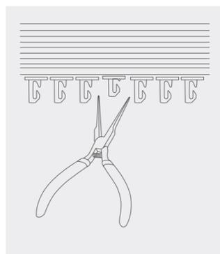
If not, check if any of the pegs within the headrail have been pushed in, if they have, using a pair of pliers, gently pull the pegs back out.
