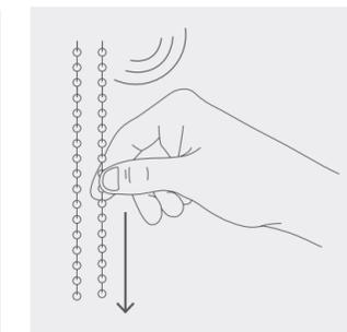
At this point you will need to pull on the chain with force. You will hear a grinding noise - this is normal.
