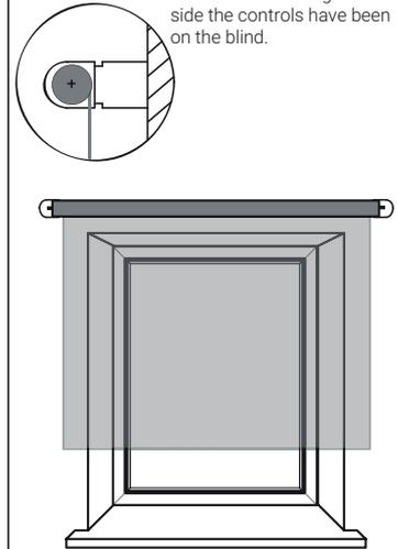
**4** The control end must be fitted first.
