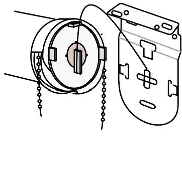
**5** Each end of the roller blind is different. One end is spring loaded as shown below. When the brackets have been installed, push the spring loaded end into the hole (in the shape of 'O'). The spring plug can push in by 1cm to give a better fit if needed.
