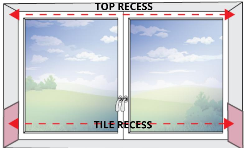
Top Recess - Tile Recess Difference: Less Than 25mm
